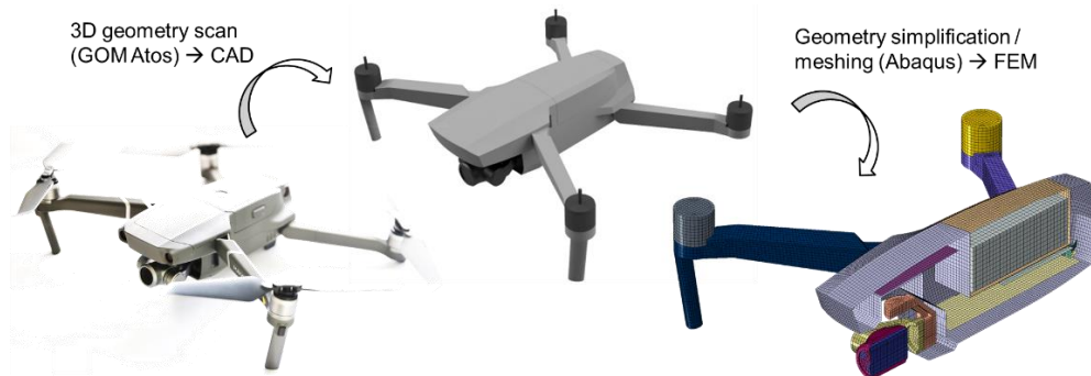
Figure 4: DJI Mavic 2 Zoom drone geometry and FE modelling
