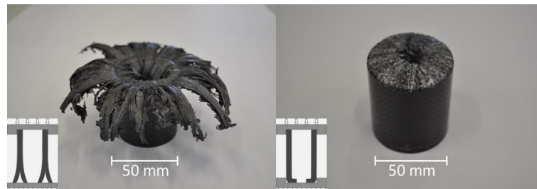
Figure [2]: Crushed CFRP tubes (1) showing outer spreading (left) and inner folding (right) based on boundary condition (a) free Crushing and (b) Inner Crushing, respectively.
