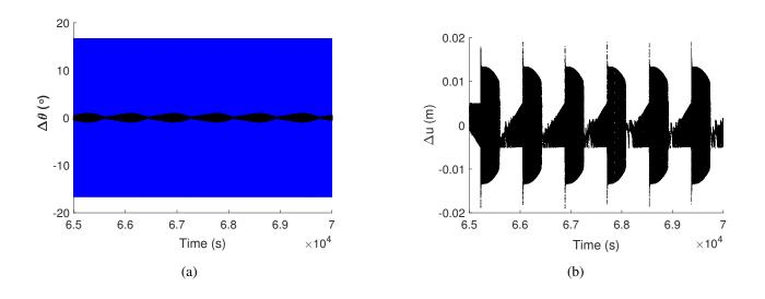
Figure 1: (a) Response of the modeled upper limb system (blue line without absorber and black like with absorber); (b) Response of the nonlinear absorber
