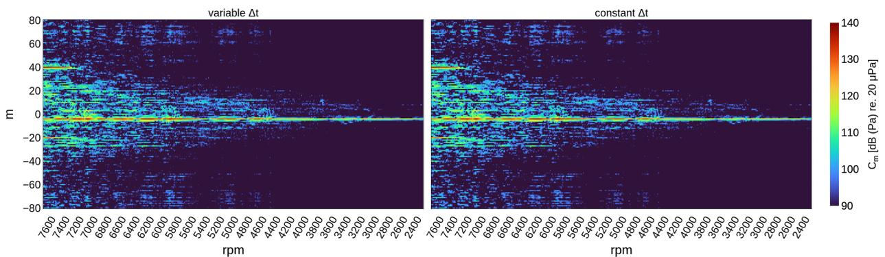
Figure 2: Map of mode amplitudes as a function of the shaft speed at the BPF2.
